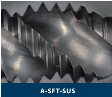
■1,000穴加工後 Cutting edge after tapping 1,000 holes
