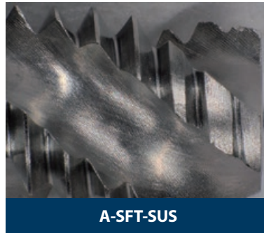
■1,000穴加工後 Cutting edge after tapping 1,000 holes
